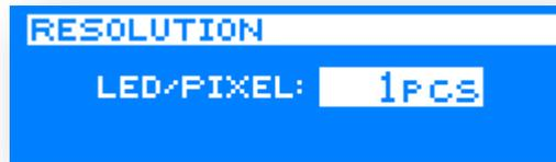
In RESOLUTION-menu you can chose how many LEDs are one pixel. You can enter values between 1 and 100.
