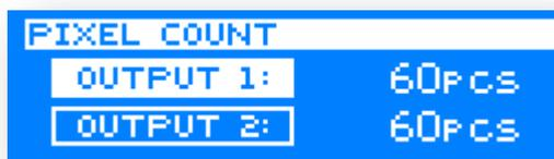
The controller has two digital outputs to control Digital Strips. In this menu you can set the amount of LEDs you have connected or you want to control at each digital output.
