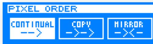
In PIXEL ORDER-menu you can chose, how the both digital outputs work together.
