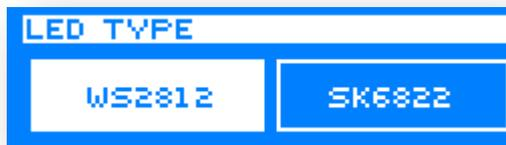
With the UP/DOWN-buttons you can chose the desired LED-type. With ENTER-button the highlighted value will be saved and the menu will be left.
